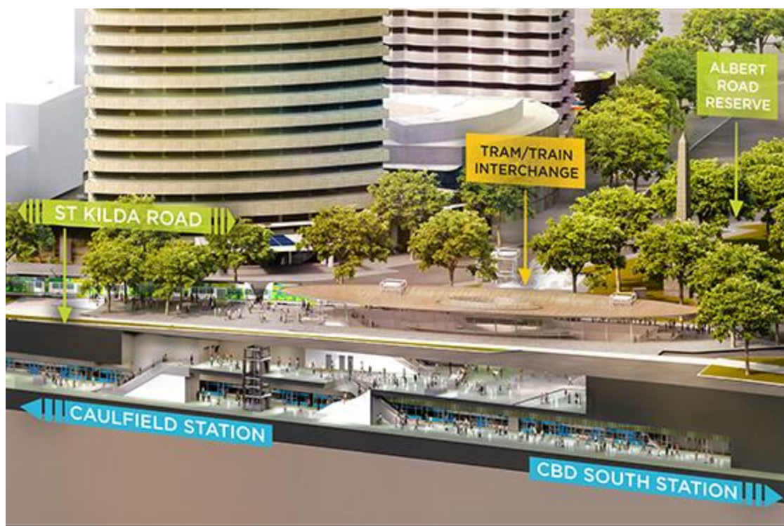
A cutaway of the new station at Domain showing platform, concourse and entrances as well as the new train-tram interchange
